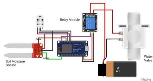
Fig 2: Circuit Diagram of the System
