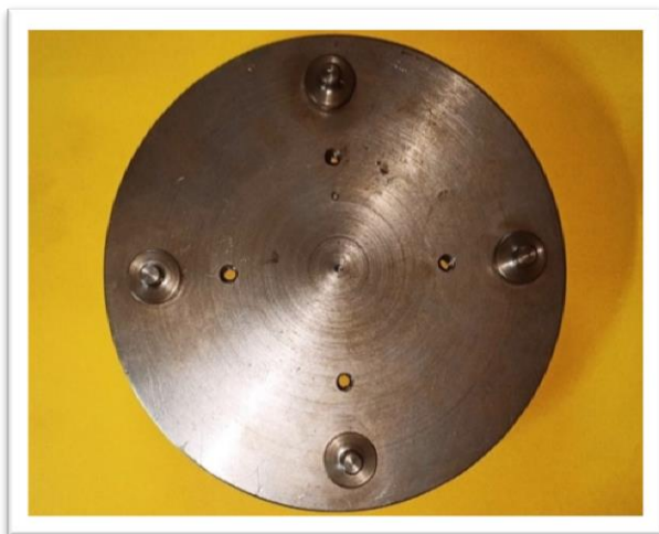
Fig- 3 Manufactured rotary Indexer with detachable fingers
