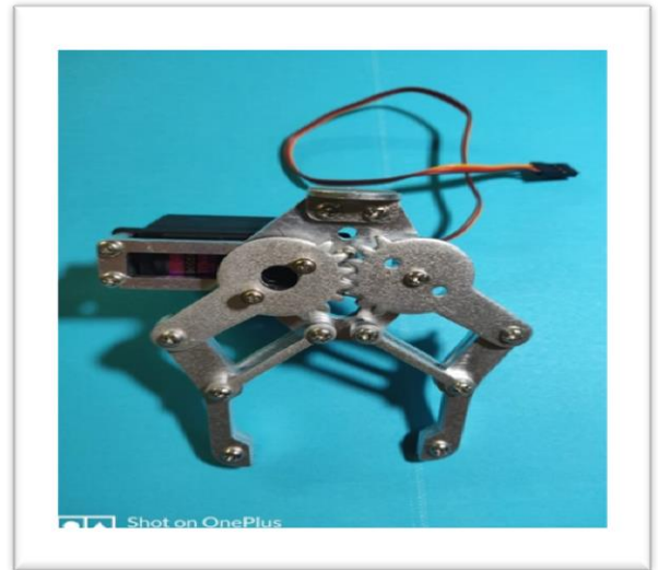
Fig- 4 Aluminum Gripper with MG996R servo
