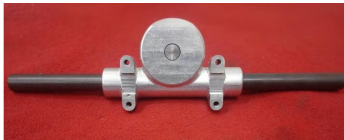
Fig -2: Manufactured Rack and pinion assembly
