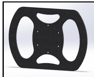
Fig. 6 Formula Student carbon fiber steering wheel
