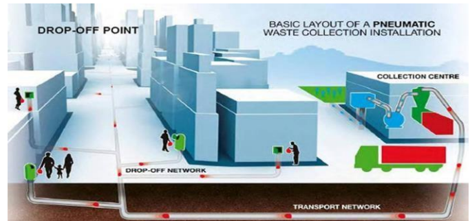
Fig. 12: Hypothetical model of pneumatic waste collection system
