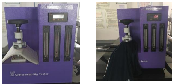
Fig 3.21. Air Permeability Test For Spacer and Sports Fabric
