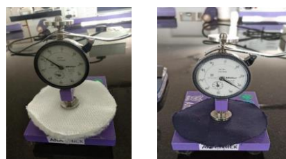
Fig-3.1.1. Thickness Test For Spacer and Sports Fabric
