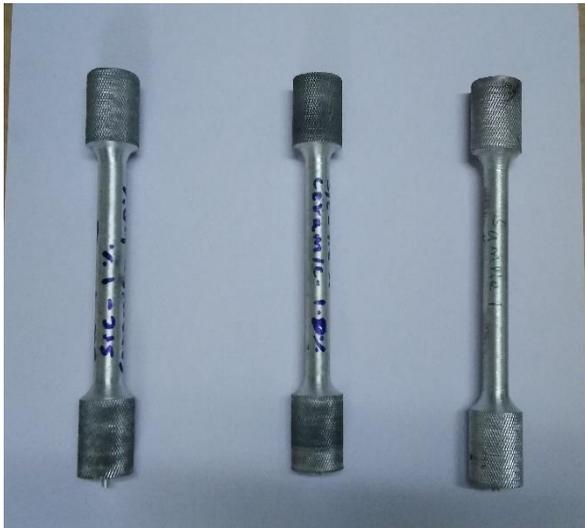
**Fig-7:** Tensile test specimen
