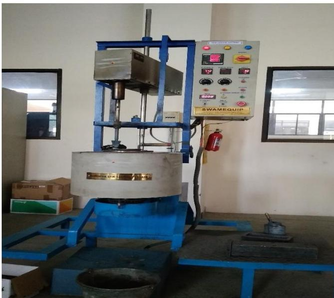
Fig- 4: Stir casting setup
