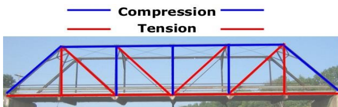
Fig-1: Truss under Compression & Tension
