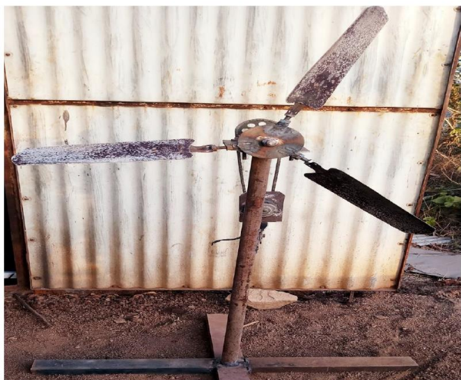
Figure 3.2 Fabricated Model Of Disk And Blade Type Wind Turbine
