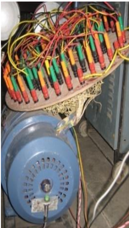
Fig-8: TPIM with outside winding connection facility
