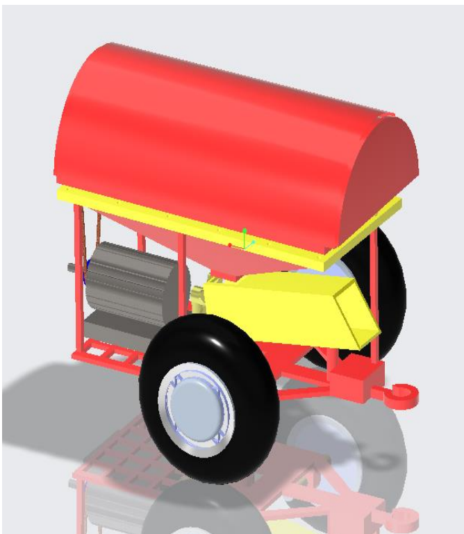
FIG NO 2: 3D PICTURE OF RICE THRESHING MACHINE
