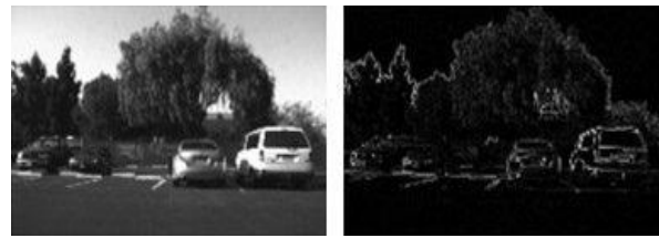
Fig 3: Image segmentation using the Sobel method.
