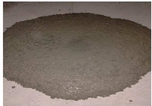
Fig -2: Flow of SCC
