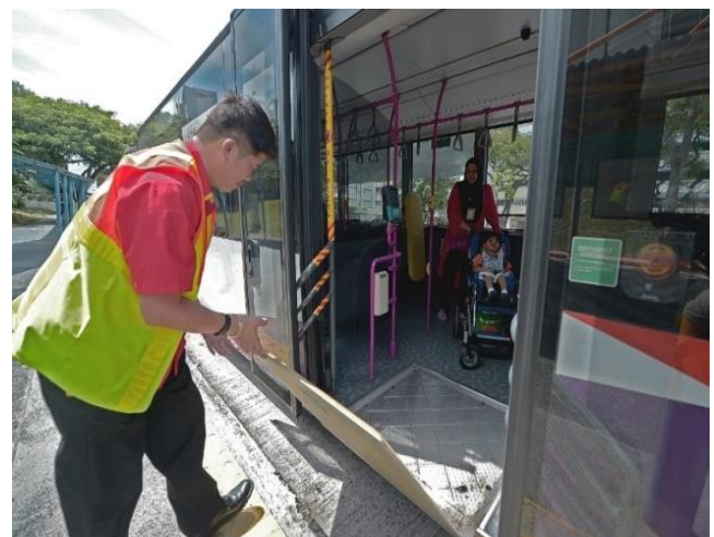
Fig3. Manual wheelchair ramp
