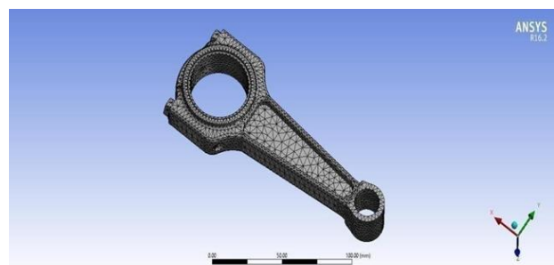
Fig 1: Meshed connecting rod showing the various elements and nodes of the mesh
