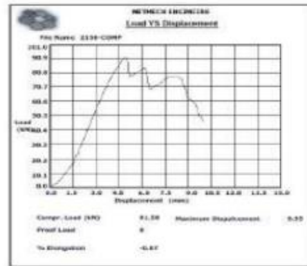
Fig 3 Load-Deflection plot of Compression test
