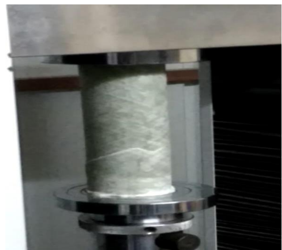
Fig 2 GFRP pipe under Compression test
