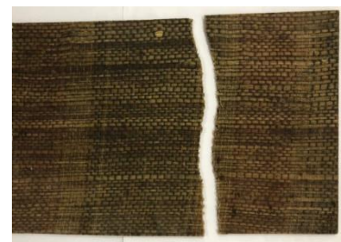
Fig - 4: Image showing material after Critical Buckling load
