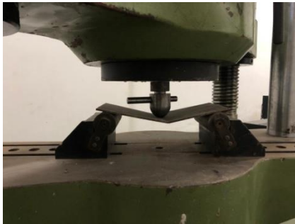
Fig - 6: Image showing Maximum Bending load of composite specimen
