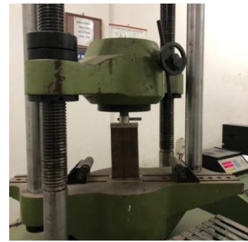
Fig -3: Image showing Buckling test of flax composite
