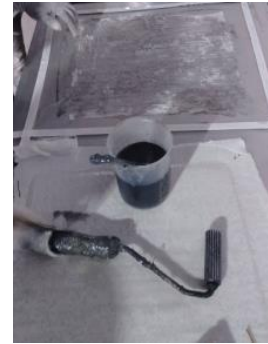
Fig -1: Fabrication of hybrid laminates by vacuum bag mould method
