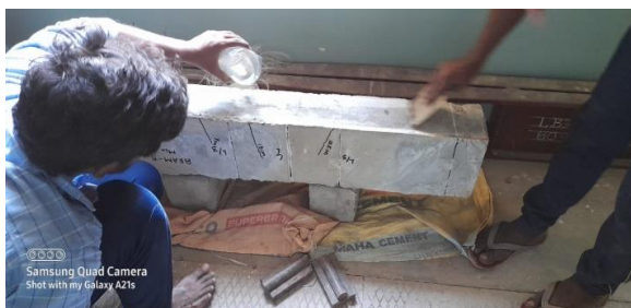
Fig- 10: Crack formed after initial loading in Beam
