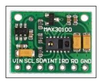
MAX30100 is an integrated pulse oximetry and heart-rate monitor sensor solution. It integrates two LEDs (IR and Red), a photo detector (Red), optimized optics, and low-noise analog signal processing to detect pulse oximetry and heart-rate signals. It is fully configurable through software registers and the digital output data is stored in a 16-deep FIFO within the device. It has an I2C digital interface to communicate with a host microcontroller.
