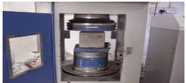
Fig. No-1 Compressive Strength Test.
