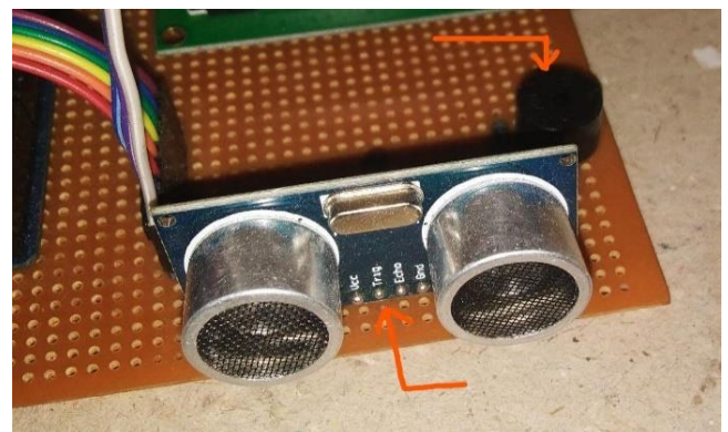
Fig5.- HCSR04 (ultrasonic) sensor and Buzzer
