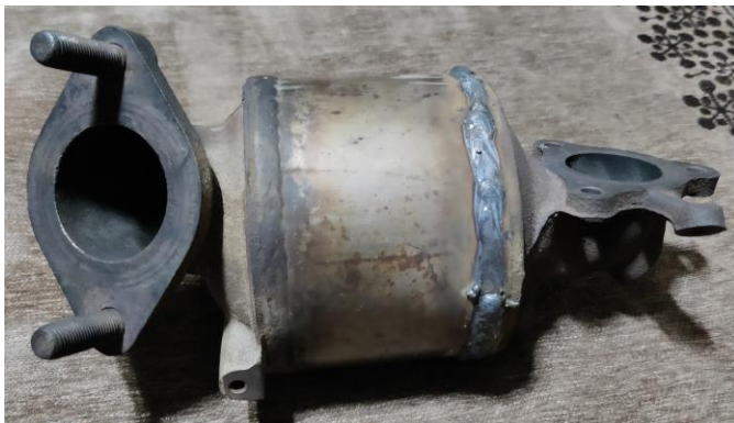
Fig -13: Argon welded modified CC
