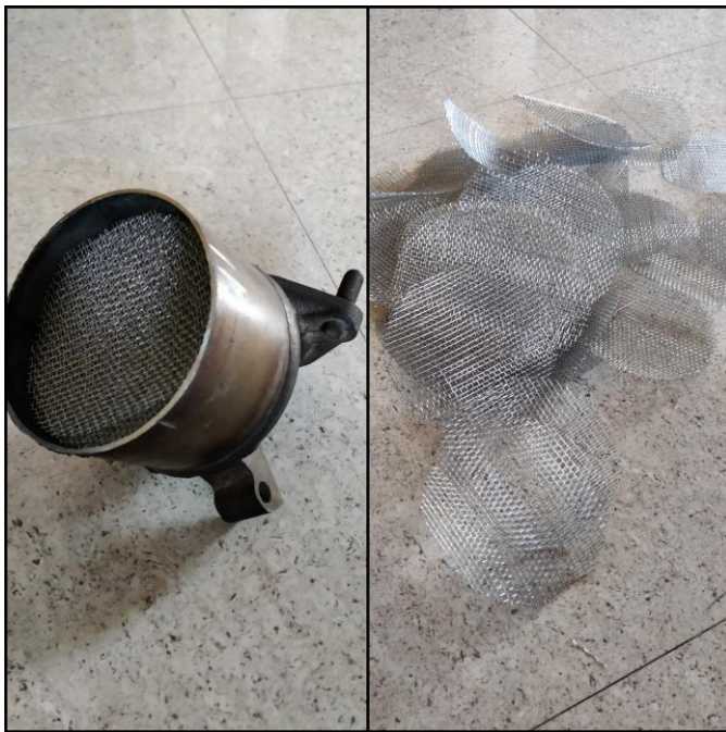
Fig -12: Zinc mesh fitted inside modified CC
