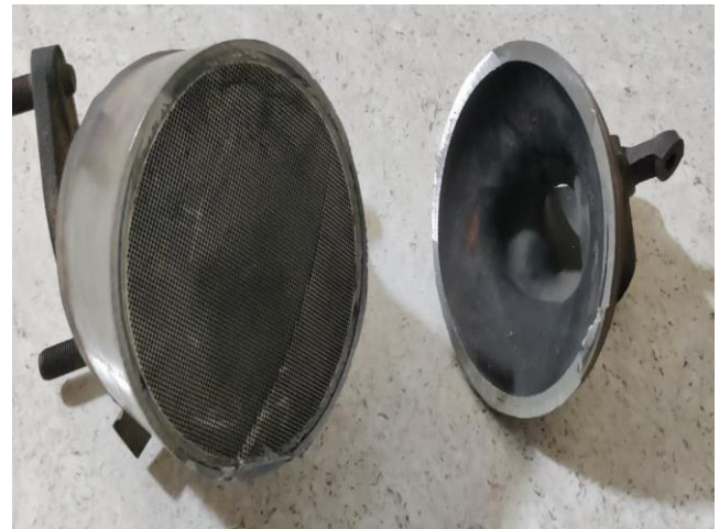
Fig -10: Conventional CC cut lengthwise
