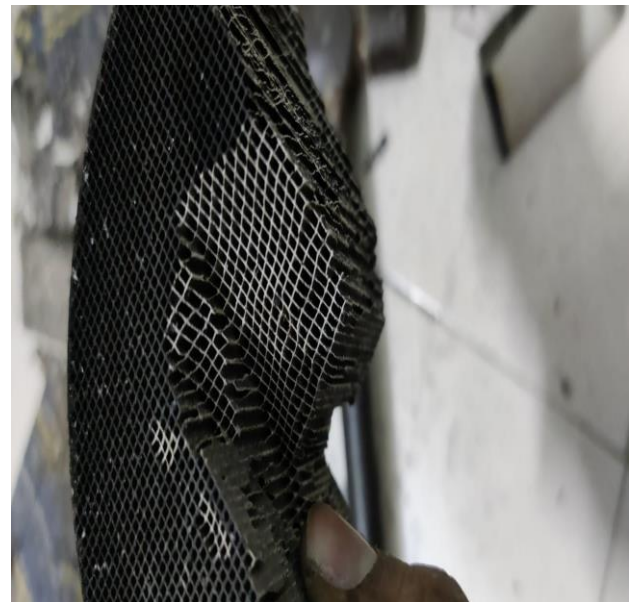
Fig -11: Honeycomb structure from conventional CC
