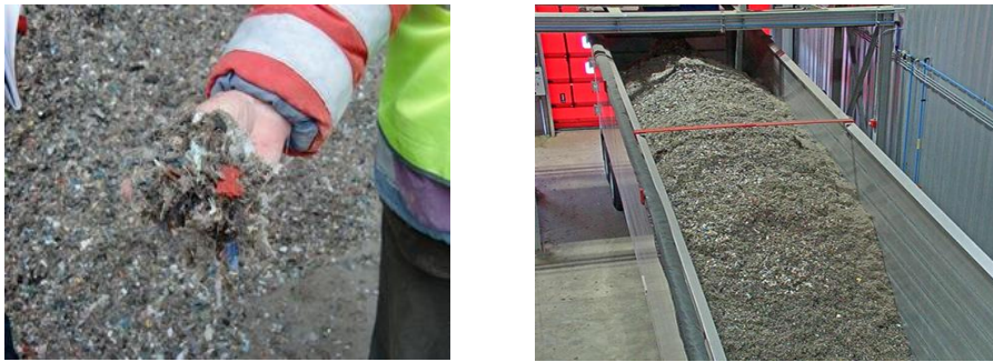
Figure - 05: SRF low quality (Left) and SRF premium quality (Right)
