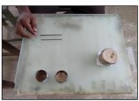
of soil on site. In addition, it also can be used to predict the consolidation properties of soil while calculating allowable bearing capacity and settlement of foundation. Plasticity index plays a crucial role as it is one amongst the two properties on which the study of swelling parameter of soil depends. Plasticity index depends on liquid limit and plastic limit of the soil
