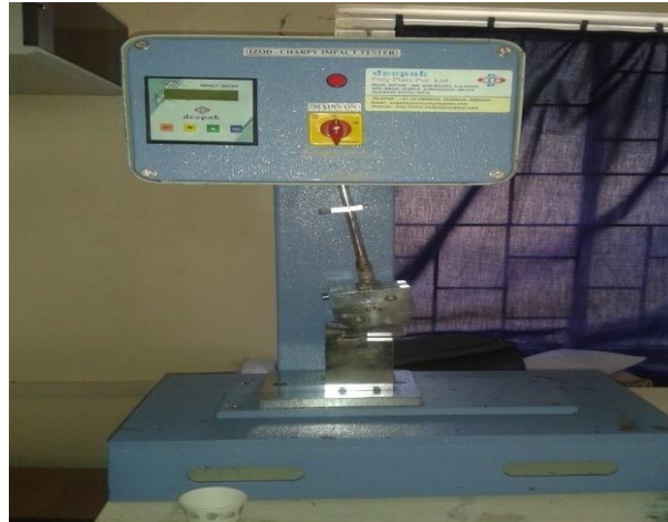
Fig-4: Impact testing machining
