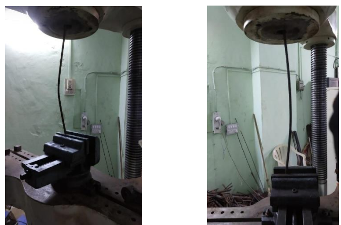
Fig -2: Buckling of Mild Steel bar Fixed at both ends.
