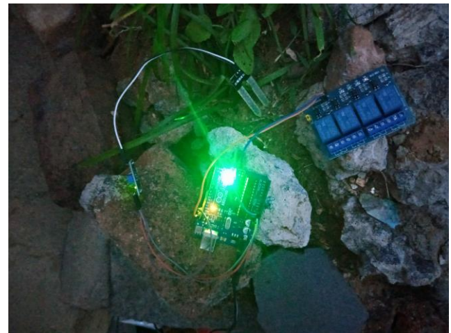
Fig.7: Prototype of Automatic Irrigation System
