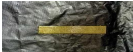
Fig 6: pH test for tap water (7.0 in pH scale)
