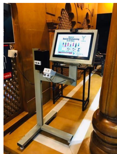
Fig 3: Face Mask Detection and Temperature Detection with access control system
