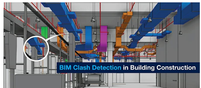
Fig -1: Clash detected between a beam and HVAC duct.
