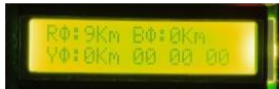
Figure-7.2: Short Circuit Fault of R-phase
