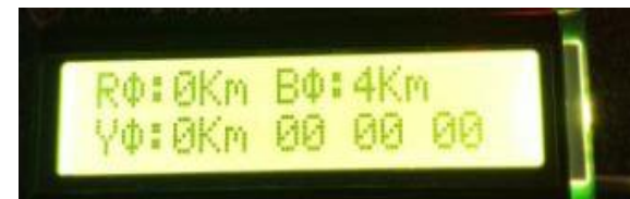
Figure-7.4: Short Circuit Fault of B-phase
