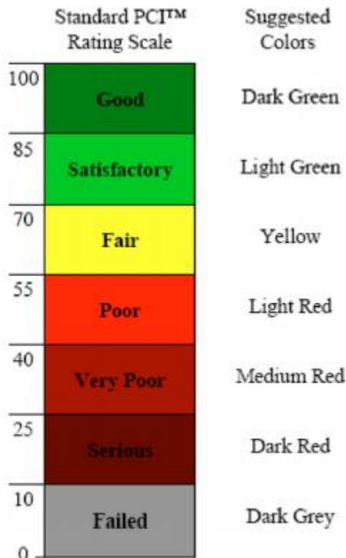
Fig. 1: Pavement Condition Index (PCI), Rating Scale, and Suggested Colors
