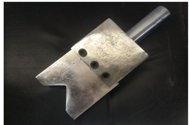
Fig: 3.2 Punch with holder Assembly
