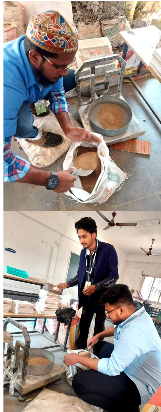
Fig -2: Batching of aggregates
