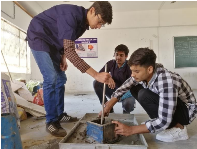
Fig -4: Casting of Cube Specimens
