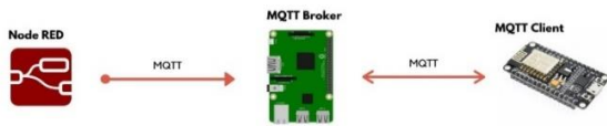
Fig. 3. This figure shows the flow of commands from node red where automation rules are programmed to the unit where the commands are executed.
