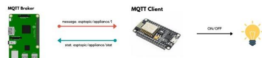
Fig. 2. This figure demonstrates the communication between the automation server (i.e. Raspberry pi) and the control unit (i.e. NodeMCU)
