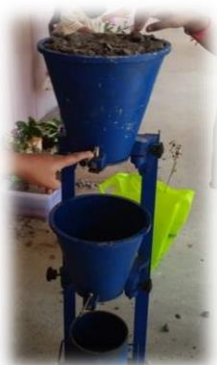
Fig 3 Compaction factor test
