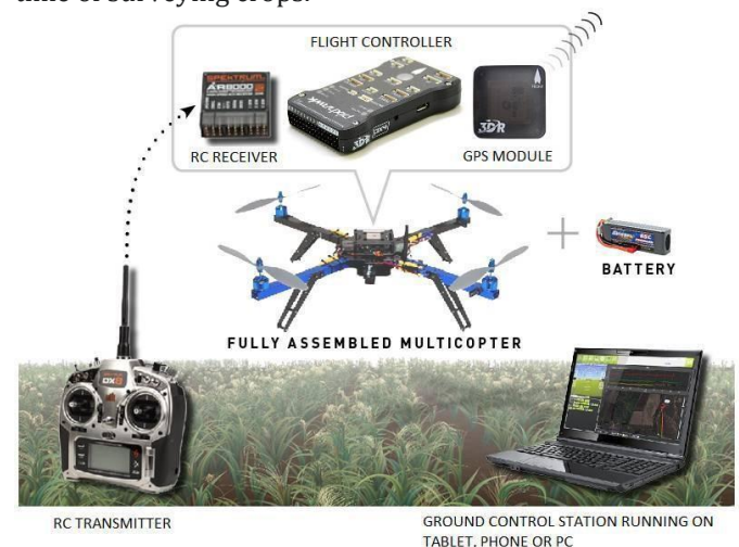
Fig -1: Control System
