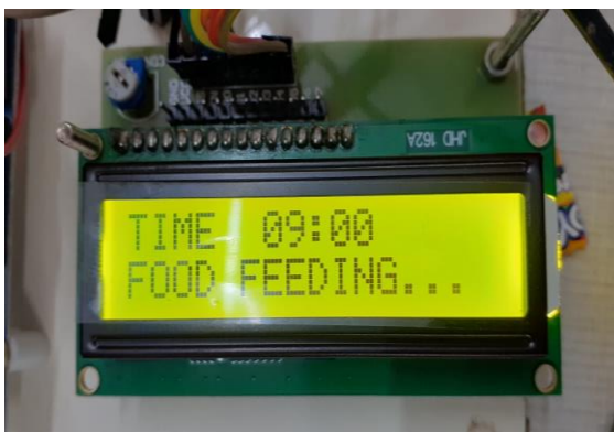
LCD Displaying the time for feeding Food and water by using RTC
