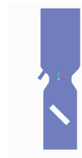
Fig-2.1: THROTTLE PLATE ANGLE – 45°
