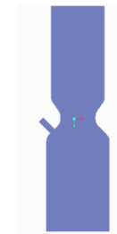
Fig-2.1: FUEL DISCHARGE NOZZLE ANGLE – 45°
