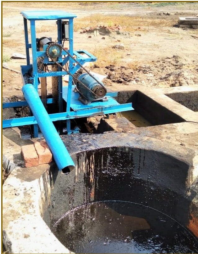
Fig -10: Assembly cum installation of full-fledged skimmer
