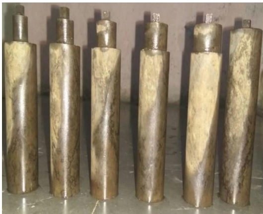
Fig. 2 H13 tools fabricated with shoulder diameters increasing from 13 mm to 28 mm with an interval of 3 mm (from left to right).
