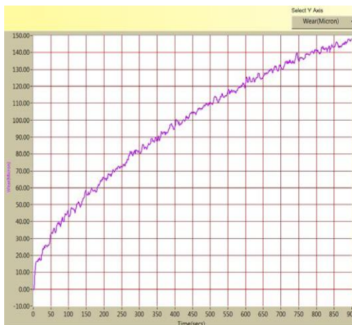
Figure 5. TIME VS WEAR
