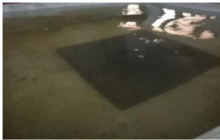
The Slab Made With Pumice Stone Fails to Float in Water
