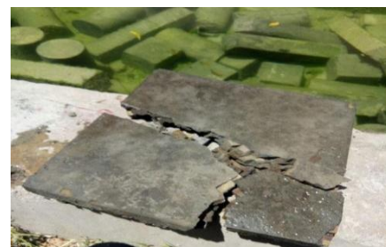
The Bond between Wood and rice husk ash is weak
