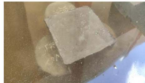
The Specimen Made With Wood Fails to Float in Water
