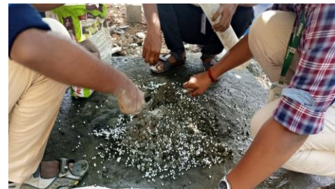
Mixing of Thermocol, Cement and Rice husk ash
