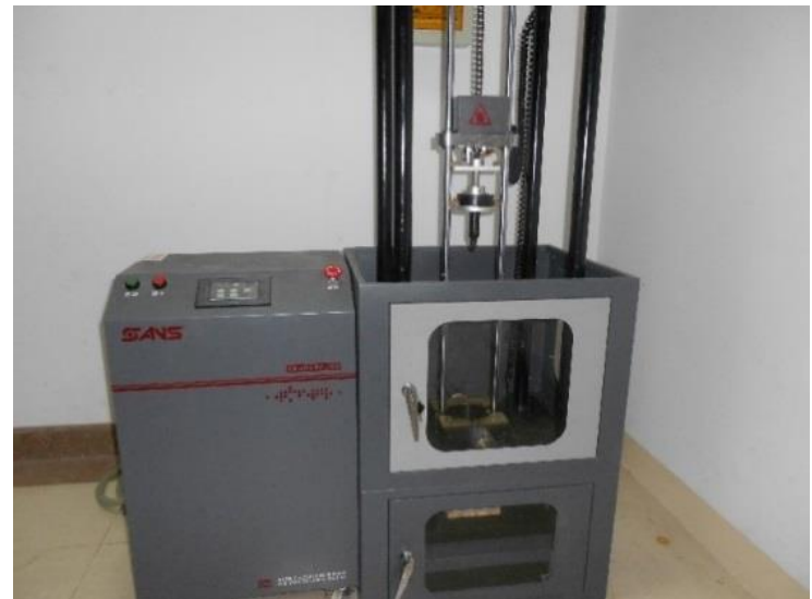
Fig -3 Falling weight impact testing machine;
