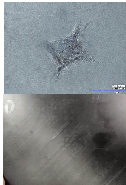
Fig -5 pointed cone punch, 30J impact view from front and back side;
