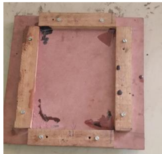
Fig -1: Die made out of medium density fiber board
