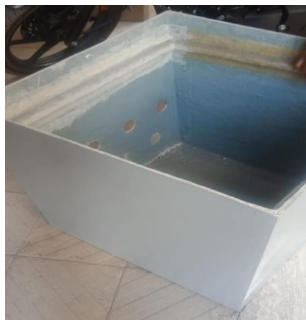
Fig -3: Holes drilled for passing of pipes through the model face
