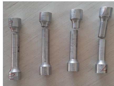
Fig: 3 Tensile test specimen after the test.
