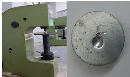
Fig:5 Brinell Hardness testing Machine and Specimen
