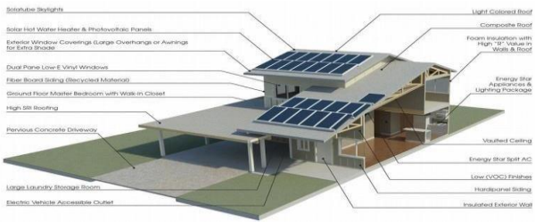
Fig. 4: Steps to reduce energy consumption
